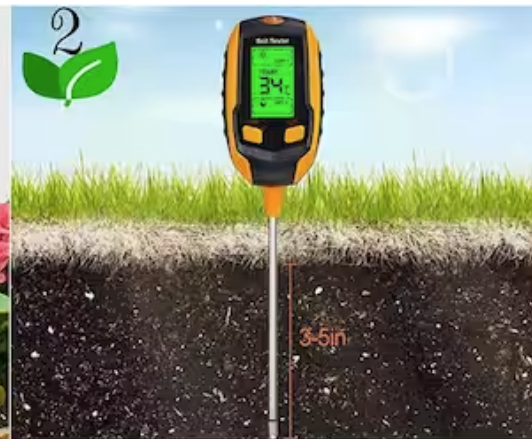
Step 2: Stick the probes into the soil 3-5 inches.
