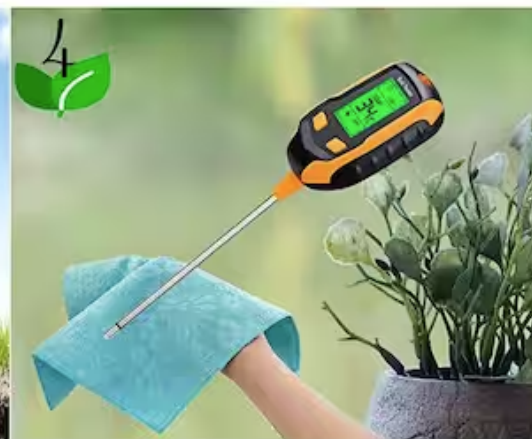
Step 4: Remove probes from soil and wipe clean after each use.
