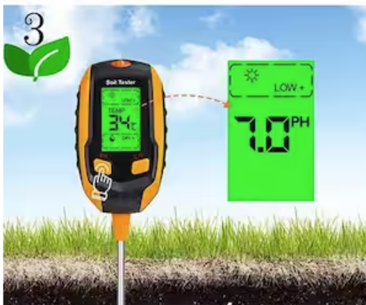
Step 3: Read the data about 10s. The pH and temperature will be toggled by pressing the pH or °C/°F button as needed.
